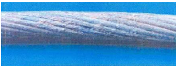
Figure 7: Zone of OPGW damaged by lightning
